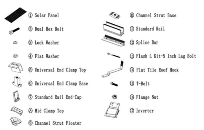
\* End Clamp, Mid Clamp and Channel Strut are pre-assembled and can be detached as top, base and other accessories such as washer and floater showing in the installation guide.
