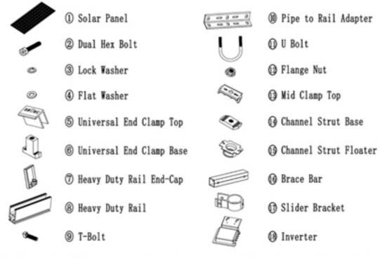
\* End Clamp, Mid Clamp and Channel Strut are pre-assembled and can be detached as top, base and other accessories such as washer and floater showing in the installation guide.
